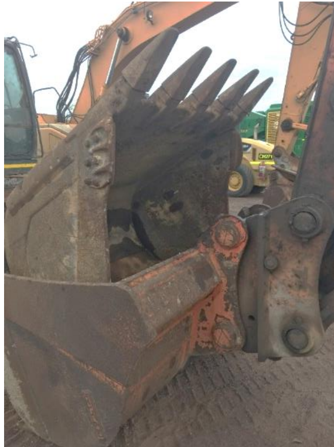
Figure 1: No Longer Acceptable - Unsecured Attachment within Large Bucket
